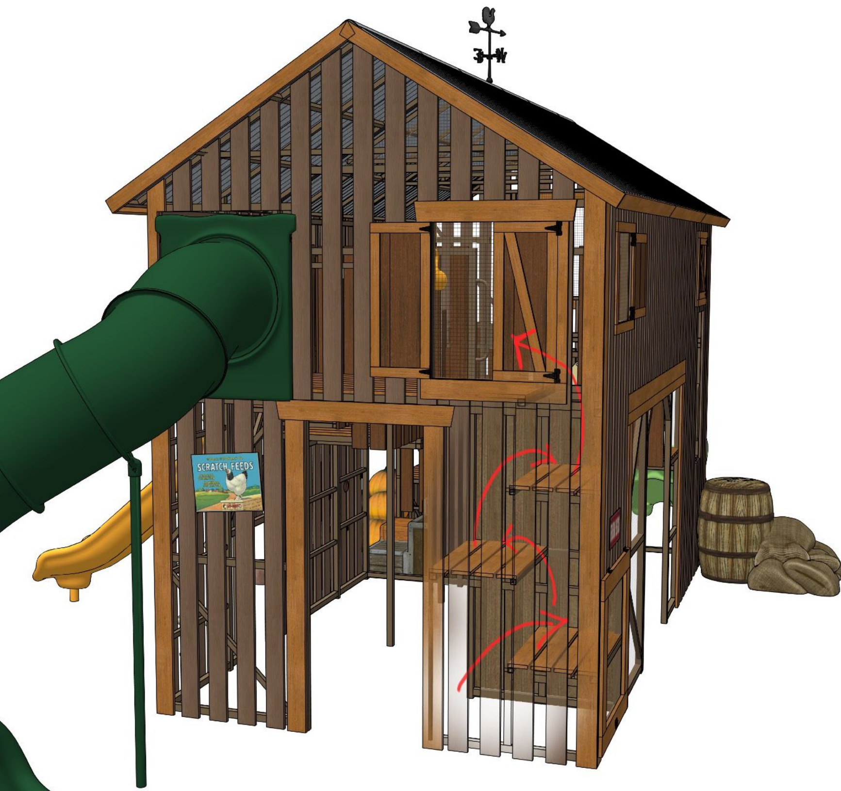
Elevator Climber Alternating platforms at 2' vertical increments
