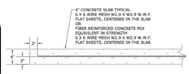
TYPICAL 4" CONCRETE SLAB DETAIL (NOT TO SCALE)
