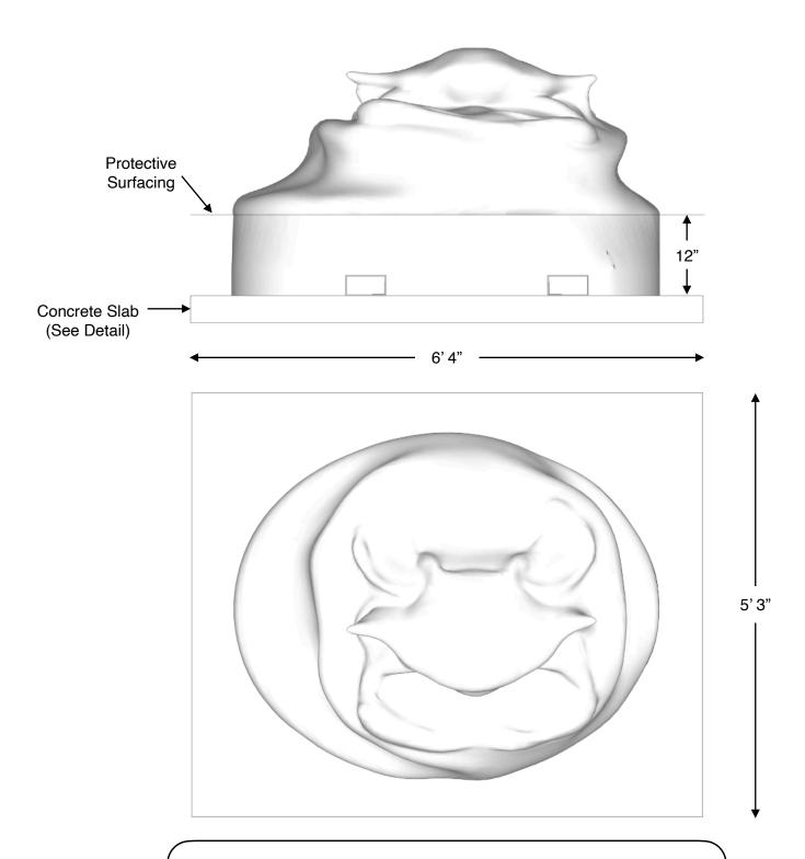
If you determine that less than 12" of surfacing is required, make sure the top of the concrete slab is 12" below the top of the protective surfacing.
