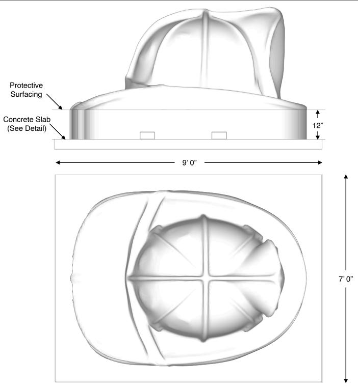
If you determine that less than 12" of surfacing is required, make sure the top of the concrete slab is 12" below the top of the protective surfacing.
