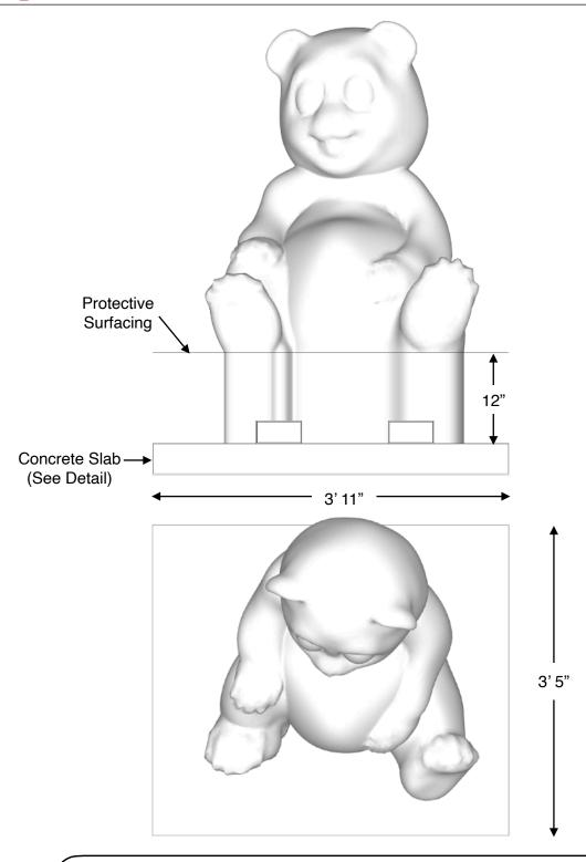
If you determine that less than 12" of surfacing is required, make sure the top of the concrete slab is 12" below the top of the protective surfacing.
