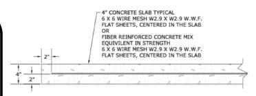
TYPICAL 4" CONCRETE SLAB DETAIL (NOT TO SCALE)
