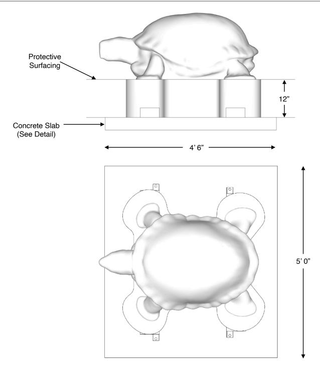
If you determine that less than 12" of surfacing is required, make sure the top of the concrete slab is 12" below the top of the protective surfacing.
