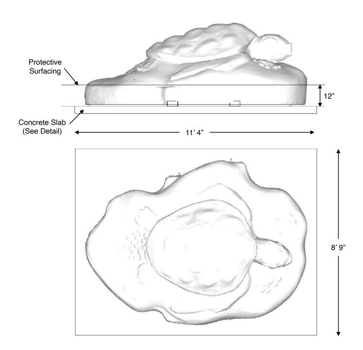
If you determine that less than 12" of surfacing is required, make sure the top of the concrete slab is 12" below the top of the protective surfacing.
