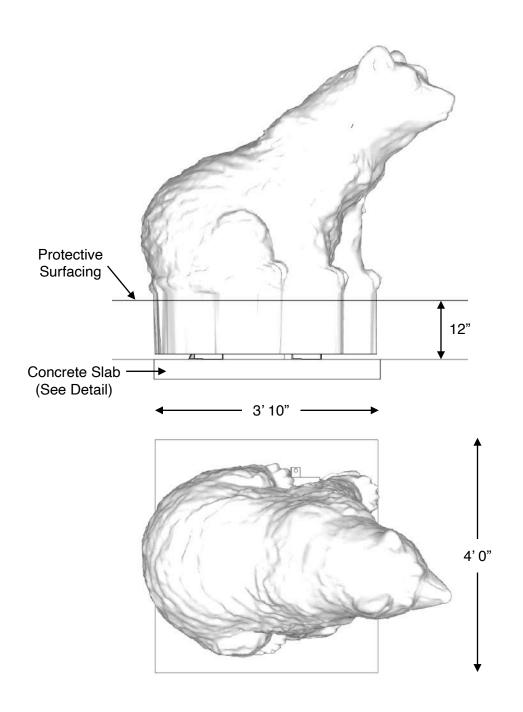
If you determine that less than 12" of surfacing is required, make sure the top of the concrete slab is 12" below the top of the protective surfacing.
